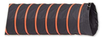
High strength sewn polyurethane coated black polyester fabric hose for high performance in lower and higher temperatures. Chemical, fuel, and oil resistant, as well as tough construction for drying, heating, & dehumidification applications. Flame retardant to UL 94V-0. 12" to 24" diameters. -60F to 400F.
